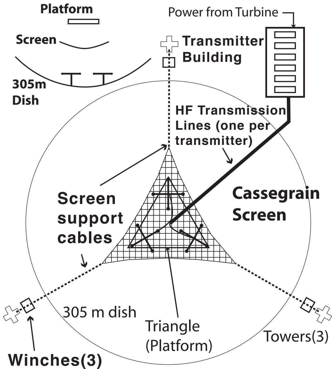
Figure 5. Schematic cartoon of the new AO on-dish heating facility. The upper left schematic shows the side-view with dipoles just above the dish surface and the convex sub-reflector mounted below the platform. The top view shows the wide-mesh Cassegrain sub-reflector and three of the six crossed-dipoles. The transmission lines are ~1000 ft in length. Figure courtesy of M. P. Sulzer, Arecibo Observatory.
